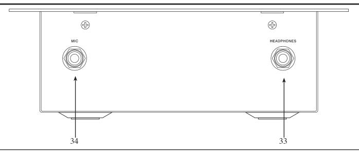
**33. HEADPHONE OUTPUT JACK -** This jack is used to connect your headphones to the mixer allowing you to monitor the cue source. Use headphones only rated at 8 ohms to 32 ohms. Most DJ headphones are rated at 16 ohm, these are highly recommended. Always be sure the CUE LEVEL VOLUME (5) is set to minimum before you put the headphones on.
